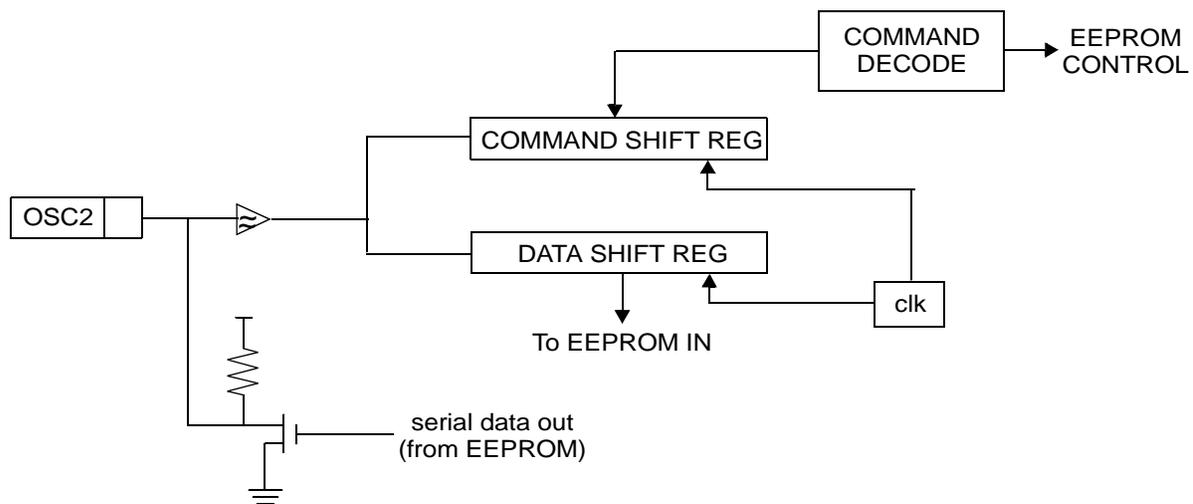
**Figure 8-5** ISP Circuit Block Diagram
