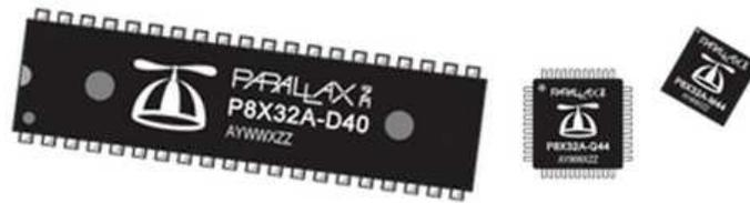
The Propeller microcontroller is pretty awesome, if we do say so ourselves. With 8 different processors (or as we call them, cogs) operating simultaneously, the development possibilities are endless!
