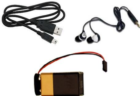
**USB A to mini B Cable & Headphones.** Used to power and program the QuickStart & listen to your radio!
