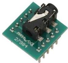
**The FM Radio Receiver Module.** The FM Radio Receiver Module uses a stereo radio tuner chip, which is how we'll get the Propeller to receive local FM radio stations.
