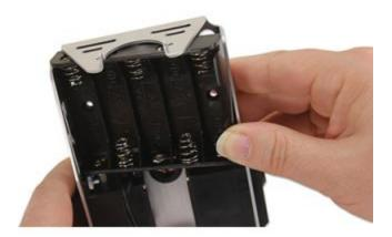
✓ Thread each nylon flat-head screw through the inside of the battery pack holes, and secure it in place with a 1" standoff.
